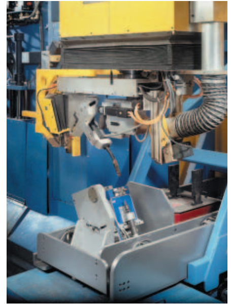
Laser-hybrid-welding head with MIG torch cleaning station
