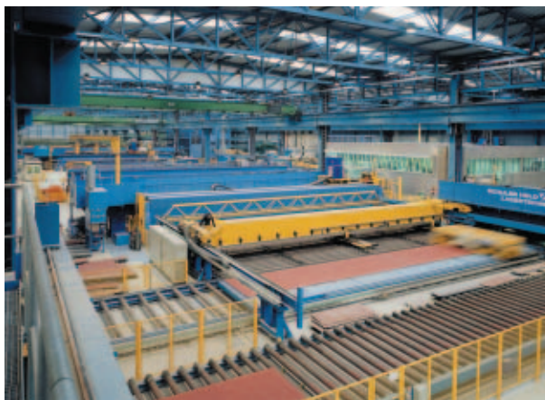
Main plate-panel-line at Meyer's new technology hall: Laser 1 on blue portal right; Laser 2 on blue portal behind yellow girder-portal
